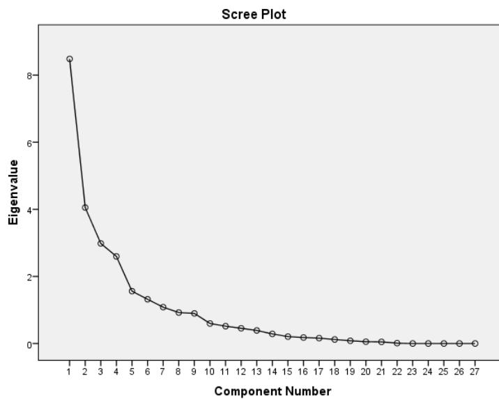
The Scree plot indicates that there are seven components which are confirmed by the initial solution extracted components by the eigen value which is greater than 1. The scree plot helps in the determination of optimal number of components. The eigen value of each component in the initial solution is plotted. The components on the steep slope are extracted. The component matrix is presented in Table 6.
